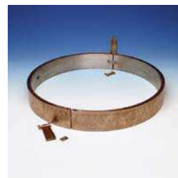
Floating cartridge This arrangement allows the sealing elements to follow the eccentric movement of worn or misaligned shafts. It is usually applied to large diameter shafts that rotate slowly.
